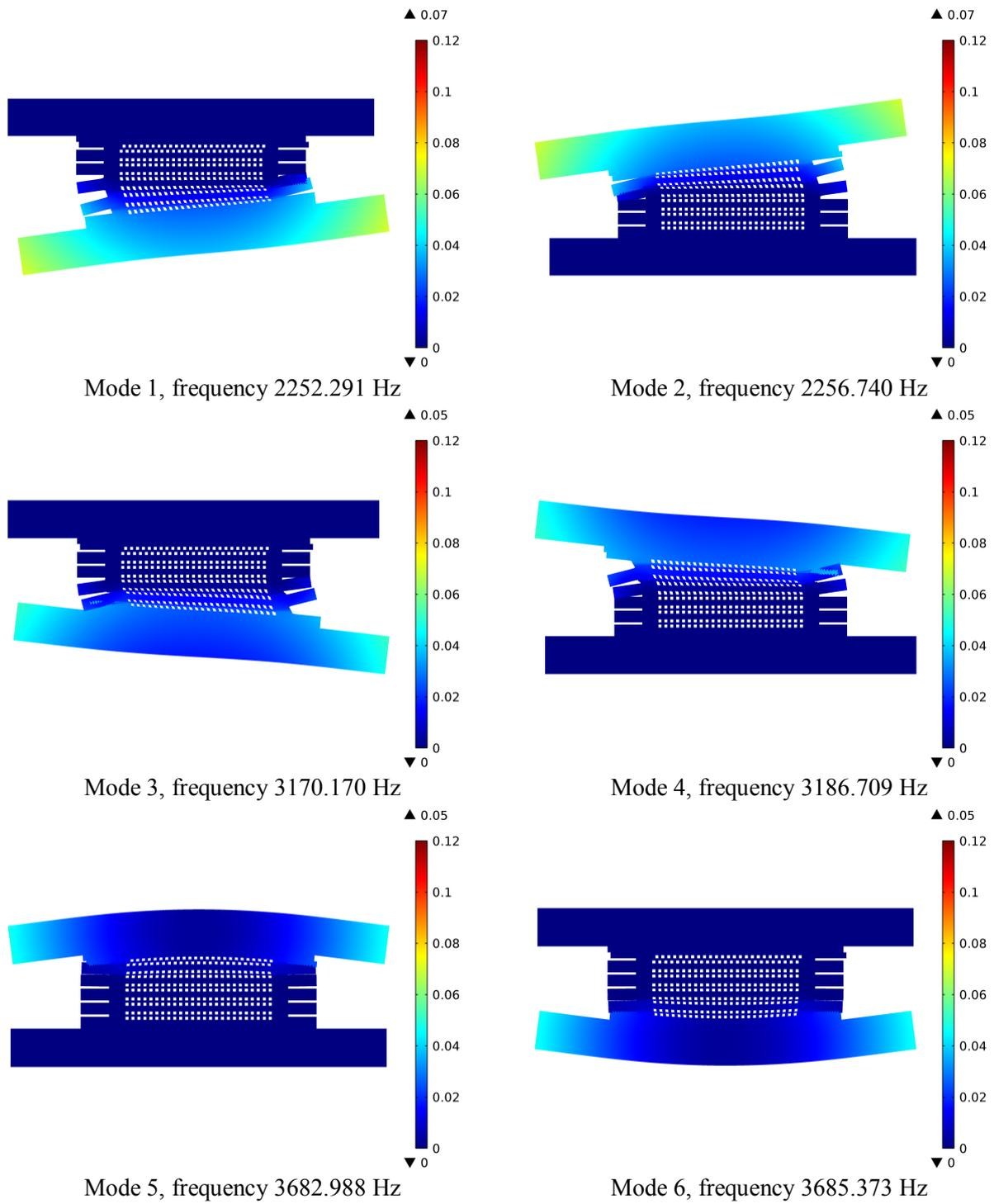
Figure 15. First six natural mode shapes with total displacement [nm]. (With assembly error: Type 1).
