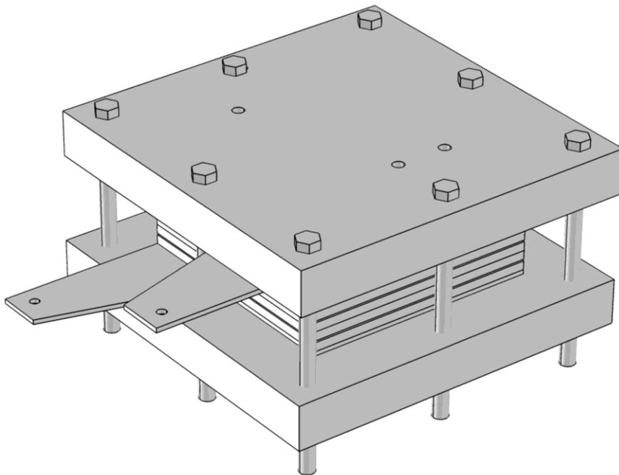
Figure 1. A PEM fuel cell stack assembly.
