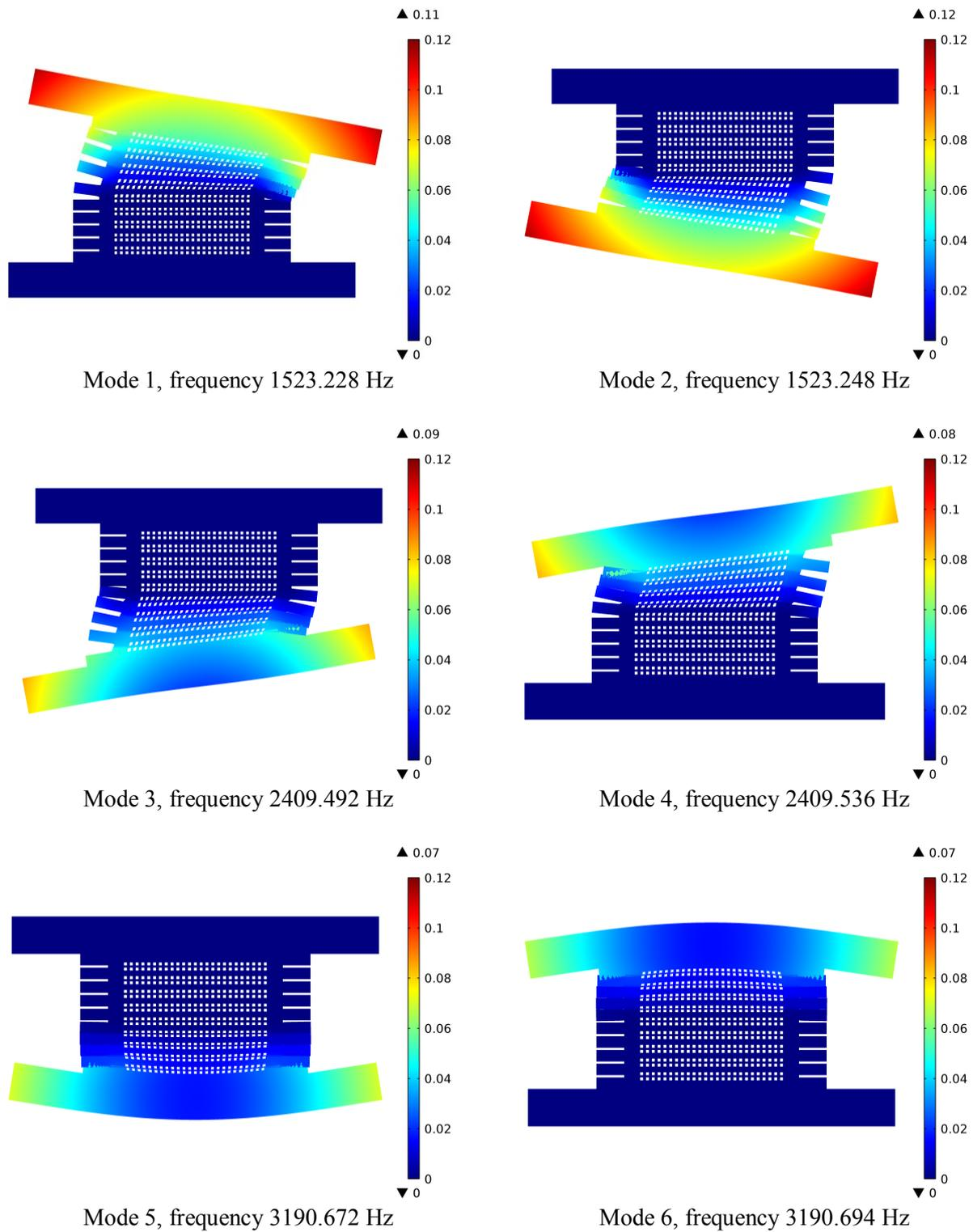
Figure 13. First six natural mode shapes with total displacement [nm]. (Number of cells in the stack = 9).
