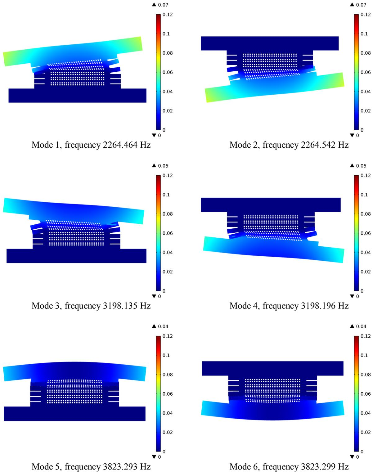
Figure 9. First six natural mode shapes with total displacement [nm]. (Current plates: Young's modulus = 209 GPa; Density = 7800 kg/m<sup>3</sup>; Poisson's ratio = 0.25).
