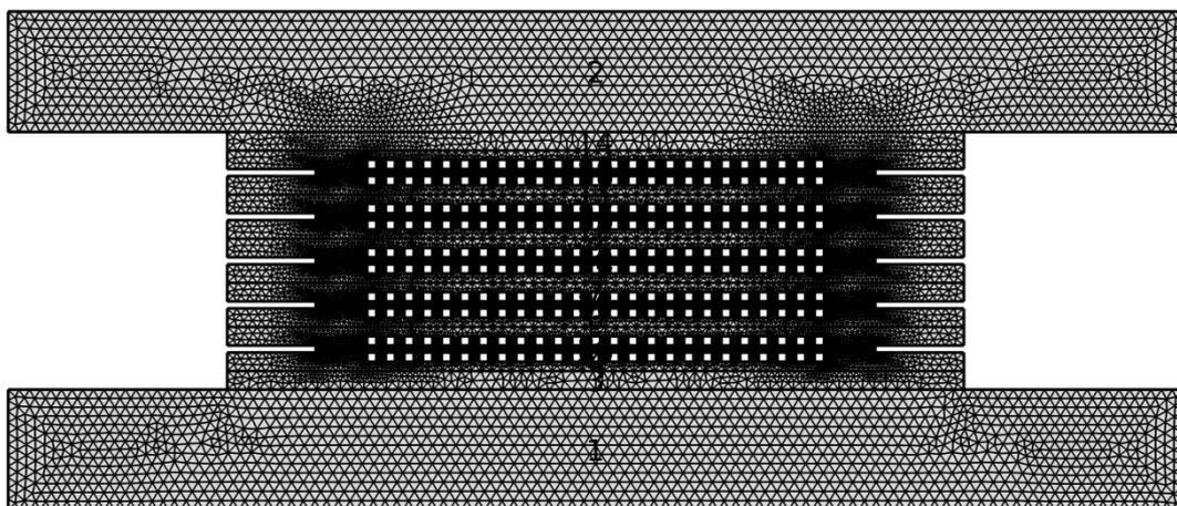
Figure 3. Computational mesh of a PEM fuel cell stack.
