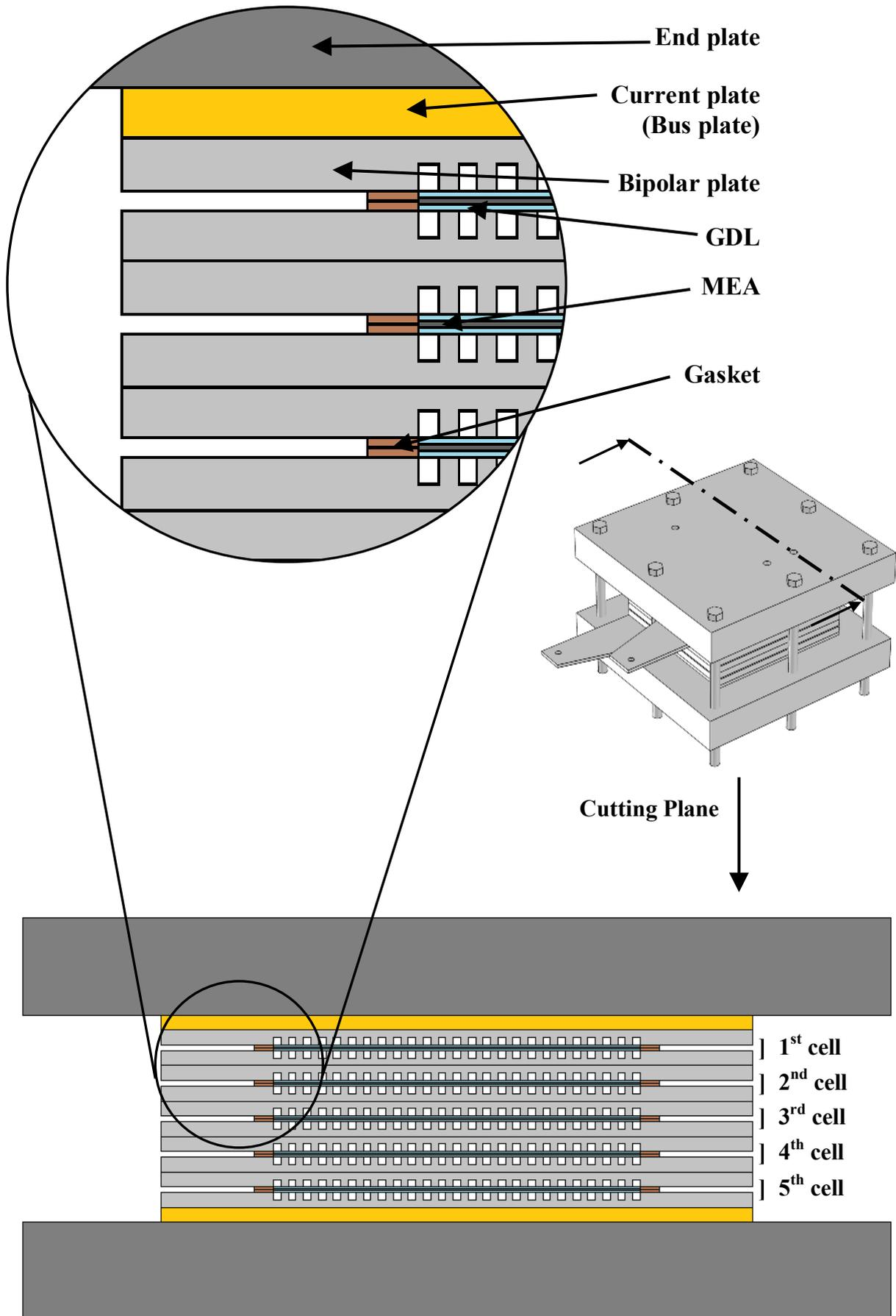
Figure 2. Description of the different stack components (Five cells).
