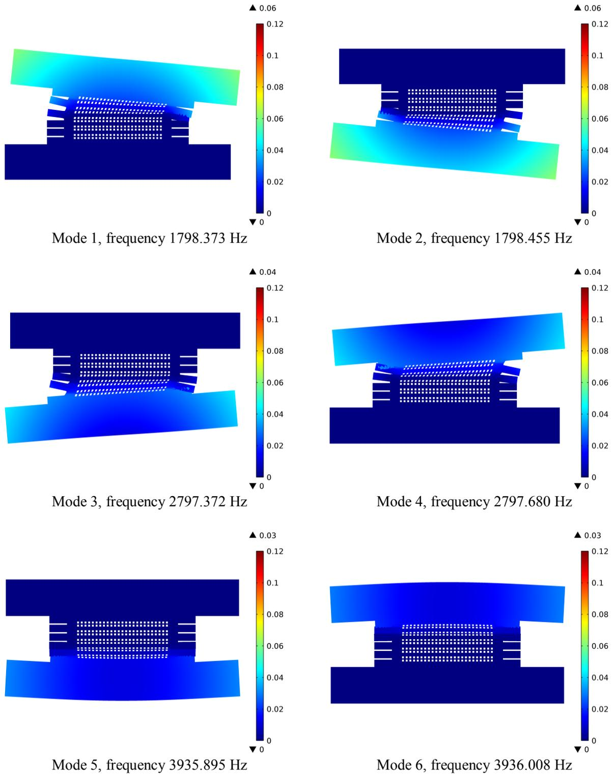
Figure 12. First six natural mode shapes with total displacement [nm]. (End plate thickness = 20 mm).
