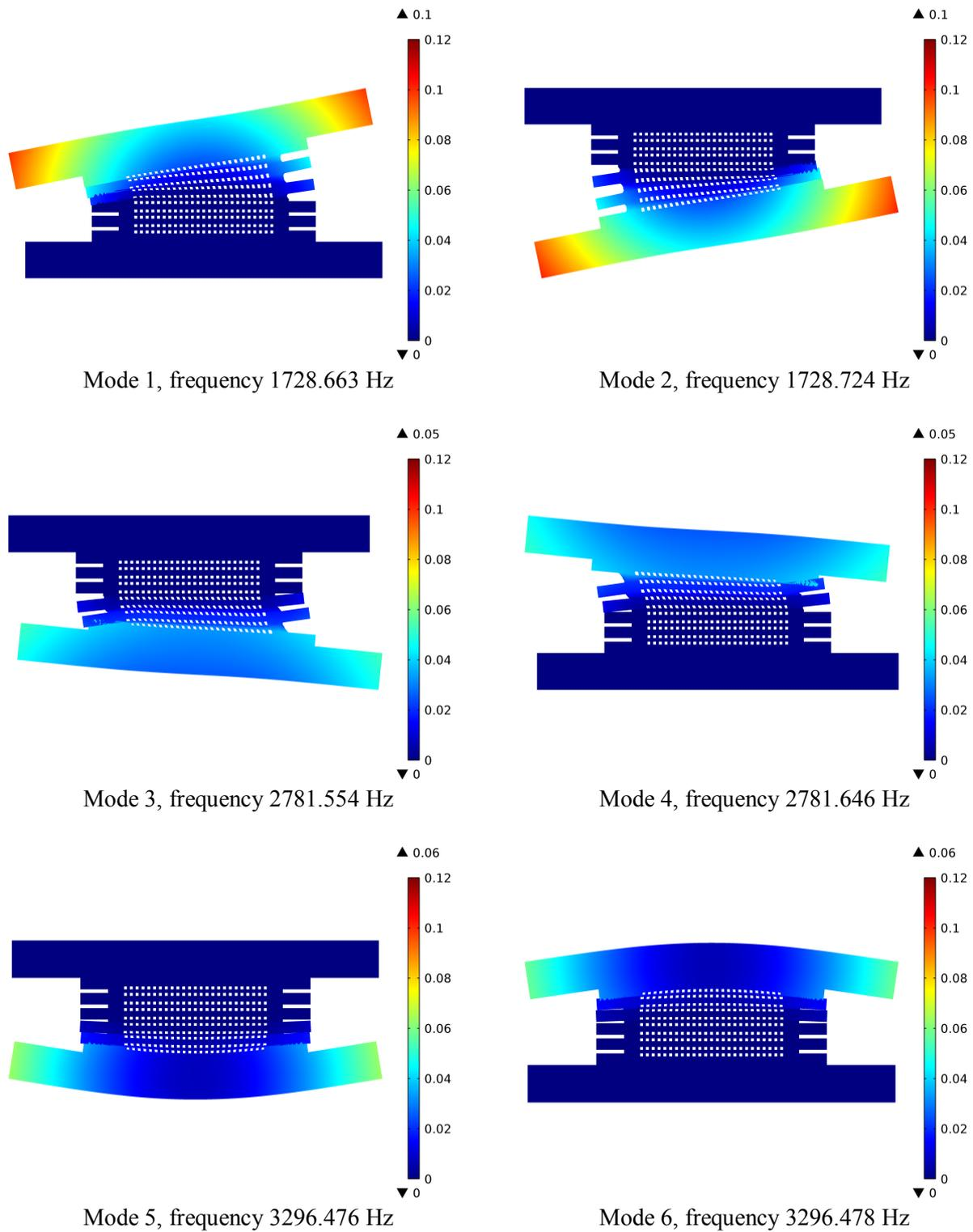
Figure 11. First six natural mode shapes with total displacement [nm]. (GDL and Gasket thicknesses = 0.5 mm).
