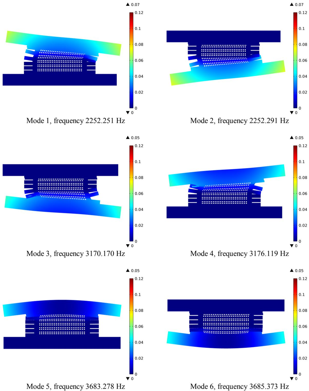
Figure 16. First six natural mode shapes with total displacement [nm]. (With assembly error: Type 2).
