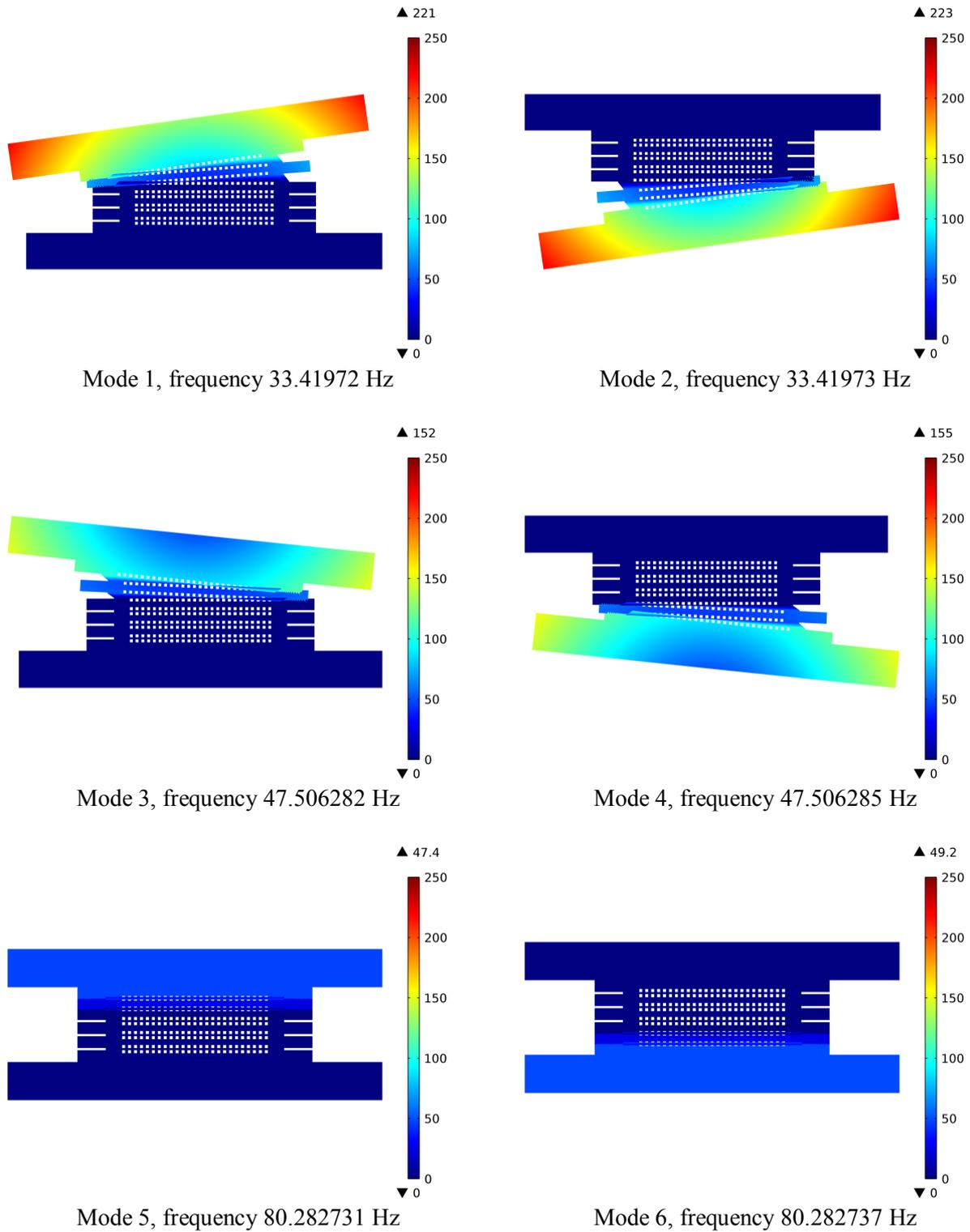
Figure 7. First six natural mode shapes with total displacement [nm]. (MEA: Young's modulus = 0.02 GPa; Density = 918 kg/m<sup>3</sup>; Poisson's ratio = 0.33).
