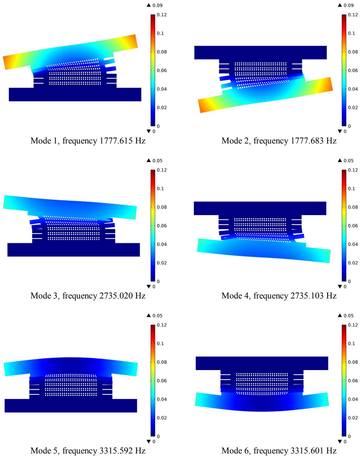
Figure 8. First six natural mode shapes with total displacement [nm]. (Gasket (Rubber (NBR)): Young's modulus = 0.1 GPa; Density = 1286 kg/m<sup>3</sup>; Poisson's ratio = 0.33).
