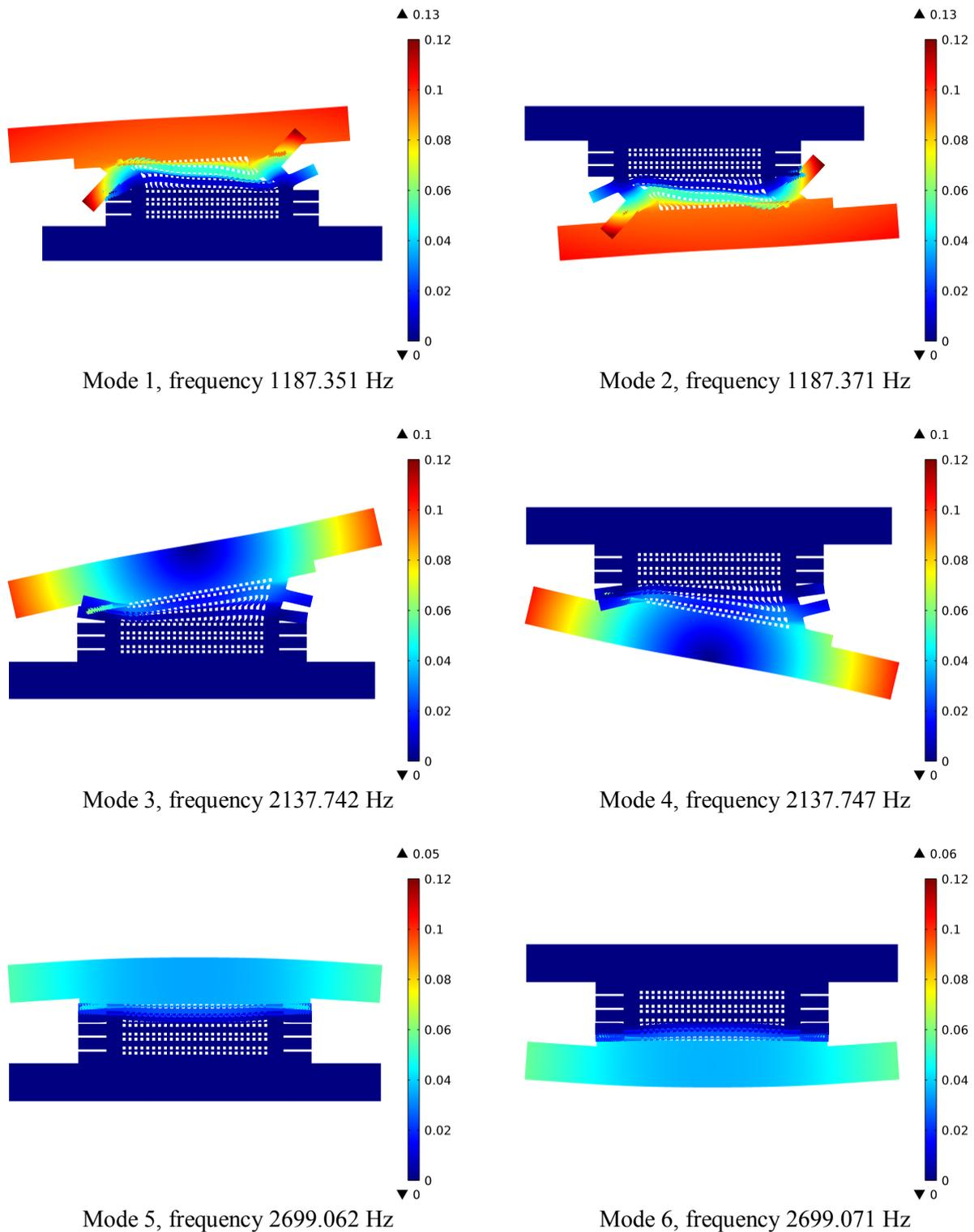
Figure 6. First six natural mode shapes with total displacement [nm]. (GDL (Toray TGP-H-030): Young's modulus = 0.0061 GPa; Density = 440 kg/m<sup>3</sup>; Poisson's ratio = 0.1).
