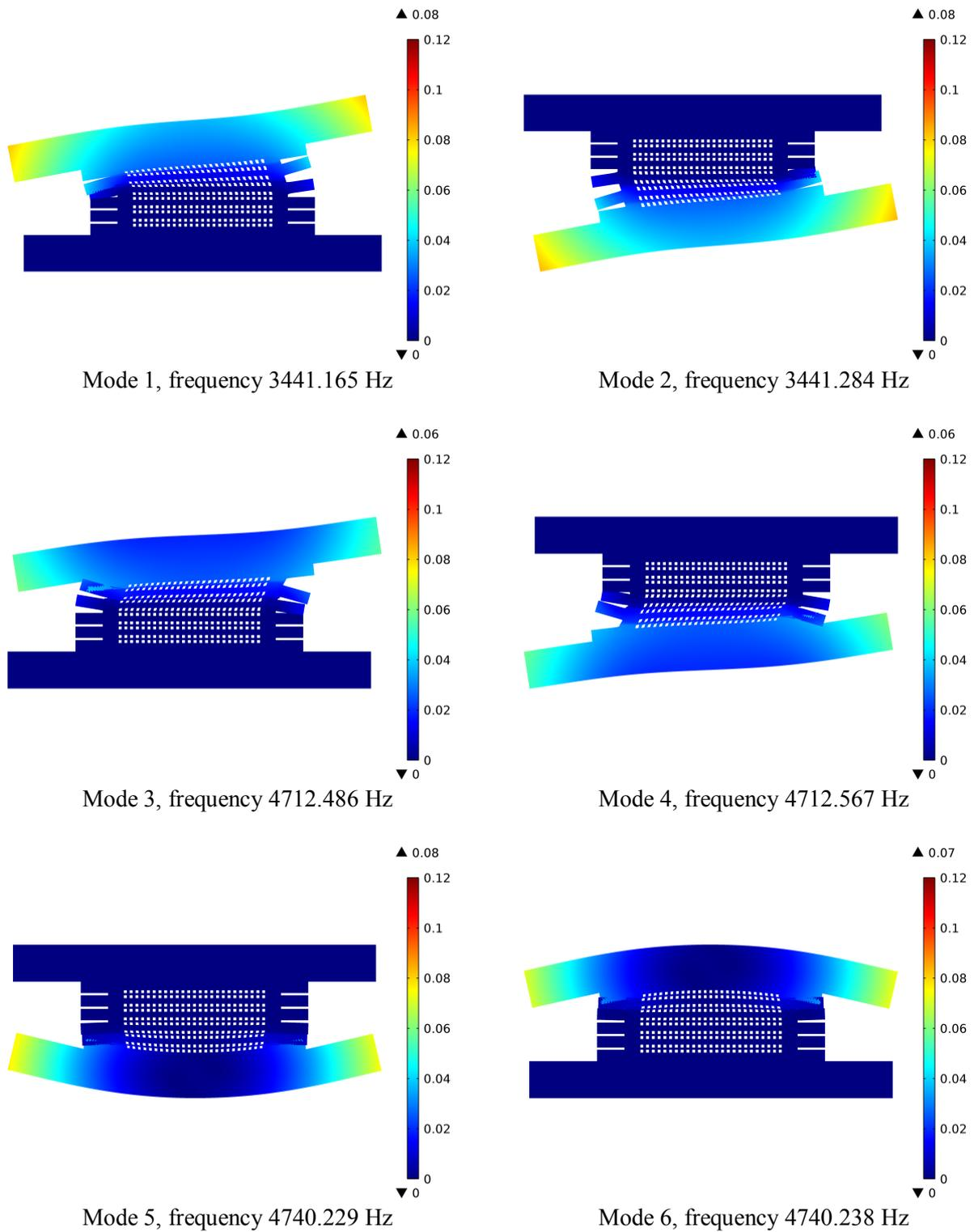
Figure 10. First six natural mode shapes with total displacement [nm]. (End plate (Aluminum): Young's modulus = 70 GPa; Density = 2700 kg/m<sup>3</sup>; Poisson's ratio = 0.33).
