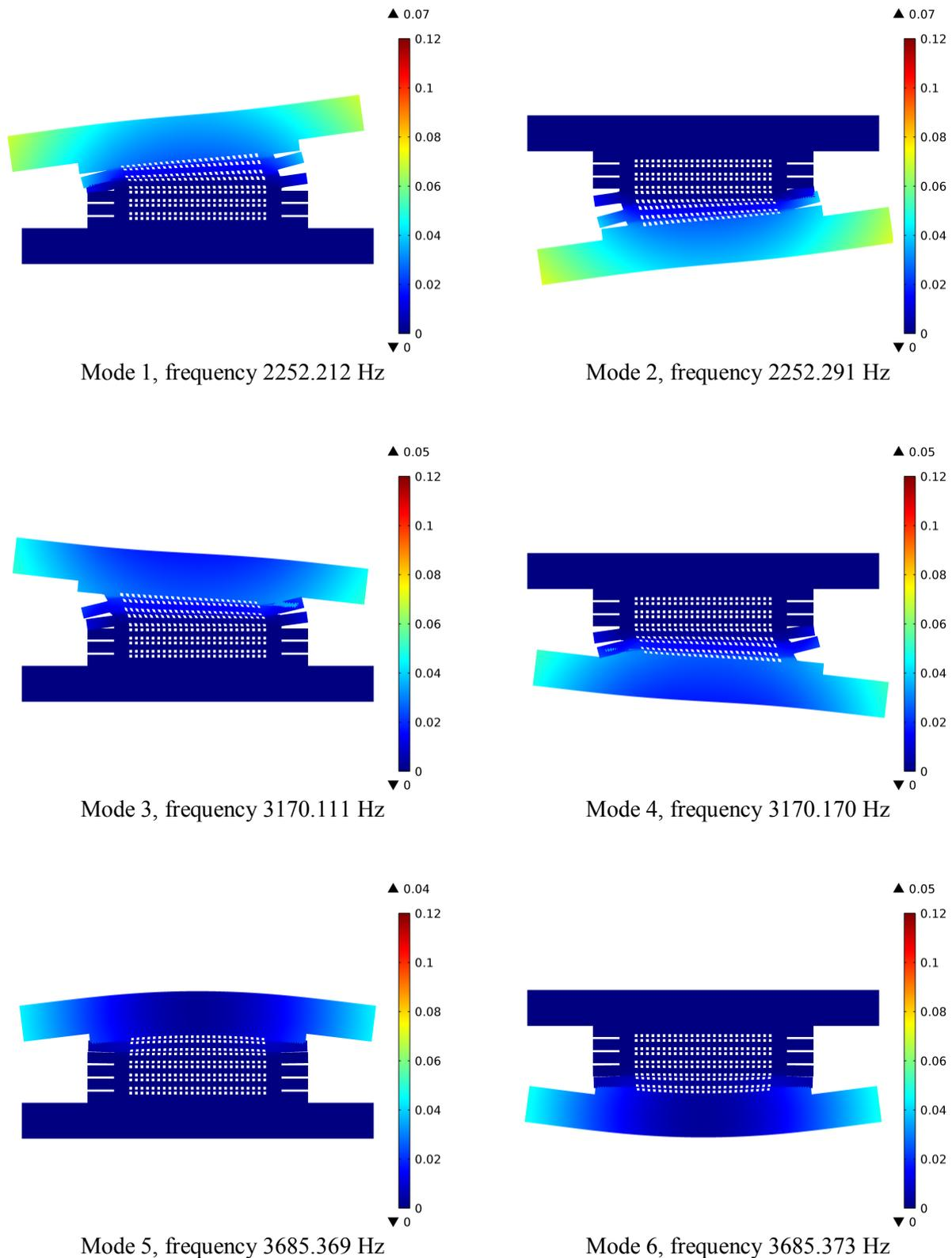
Figure 4. First six natural mode shapes with total displacement [nm].
