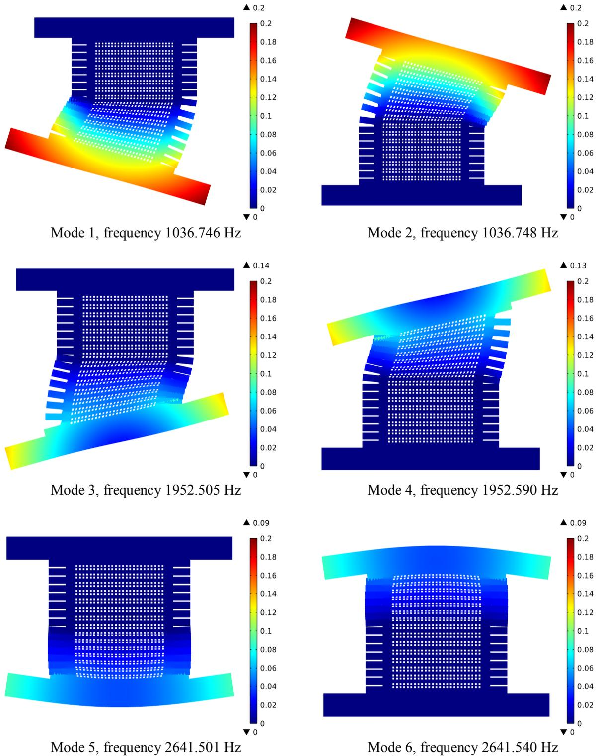
Figure 14. First six natural mode shapes with total displacement [nm]. (Number of cells in the stack = 15).
