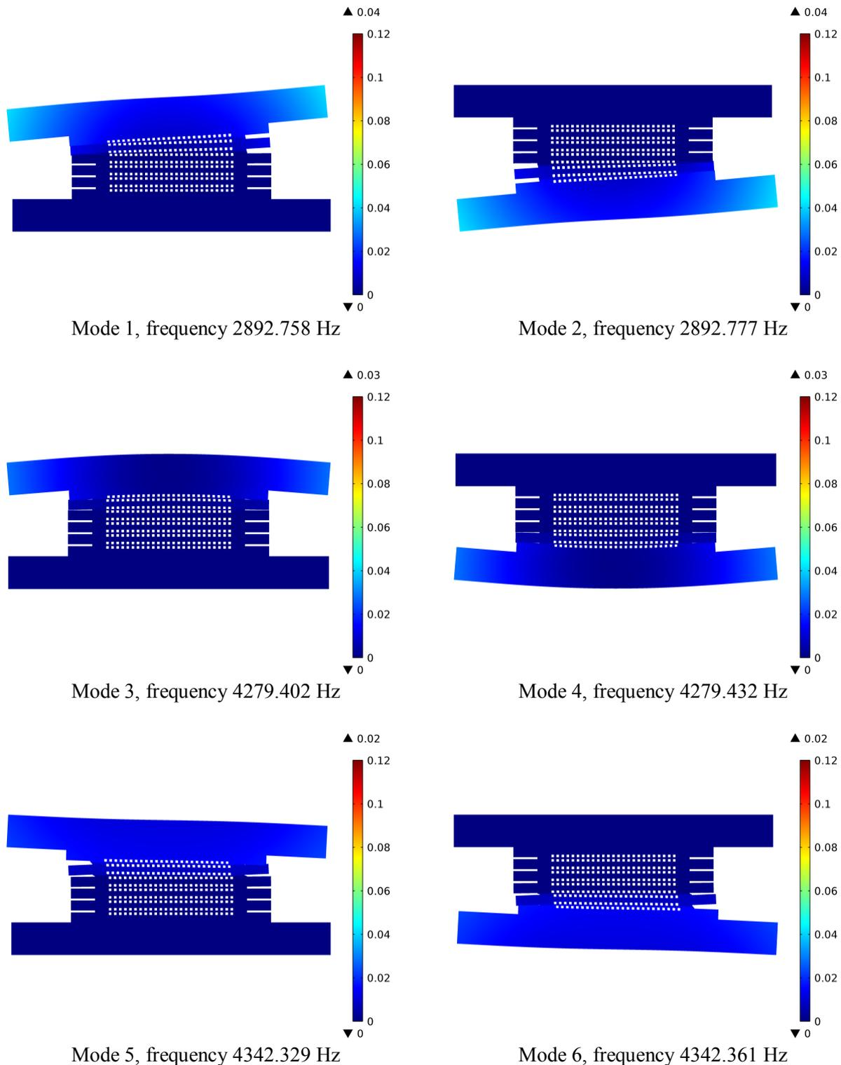
Figure 5. First six natural mode shapes with total displacement [nm]. (Metallic bipolar plate (SS316L): Young's modulus = 197 GPa; Density = 7800 kg/m<sup>3</sup>; Poisson's ratio = 0.3).
