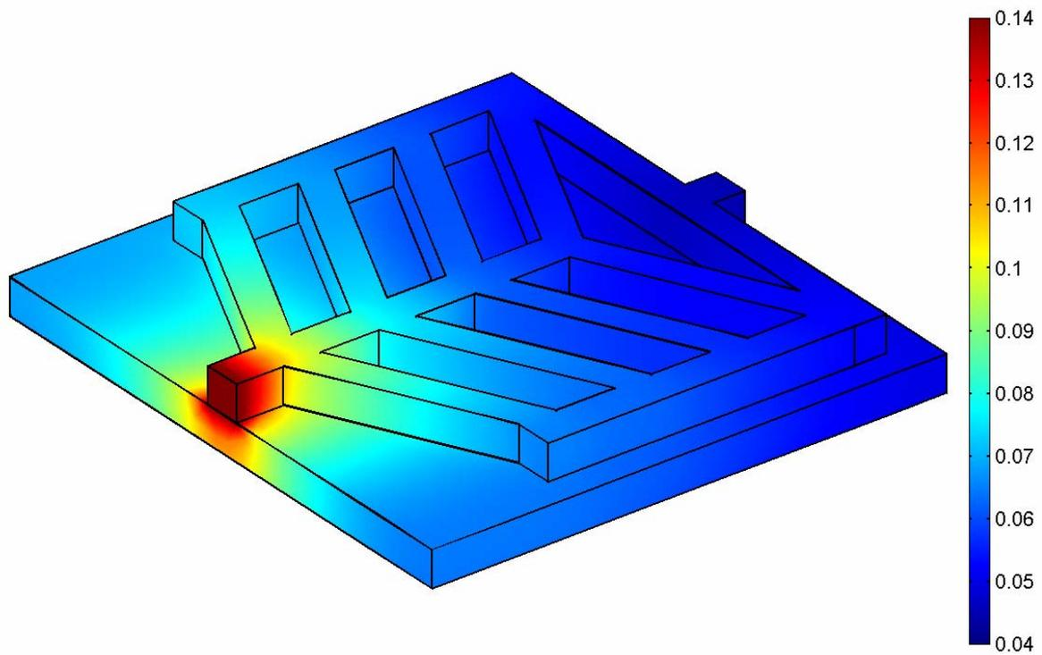
Figure 5. Oxygen weight fraction distribution.
