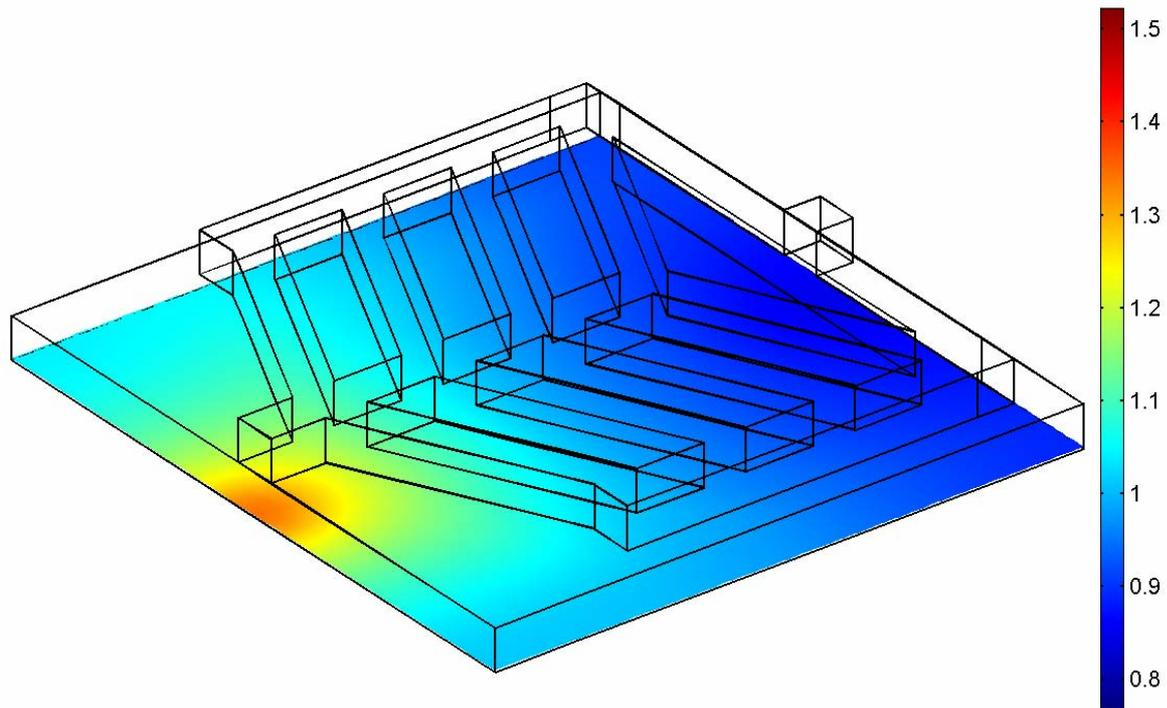
Figure 7. Dimensionless local current density distribution ( $i_c/I$ ) at cathode side catalyst layer.
