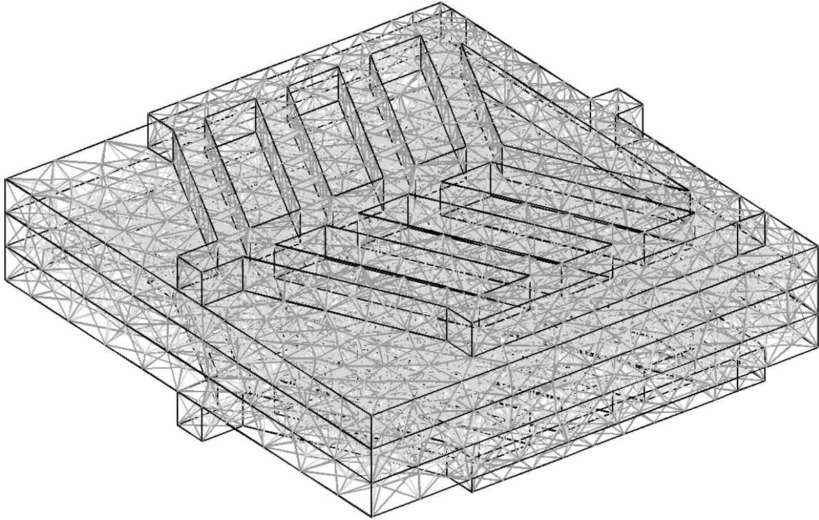
Figure 2. Computational mesh for micro PEM fuel cell with nature inspired gas flow channels.
