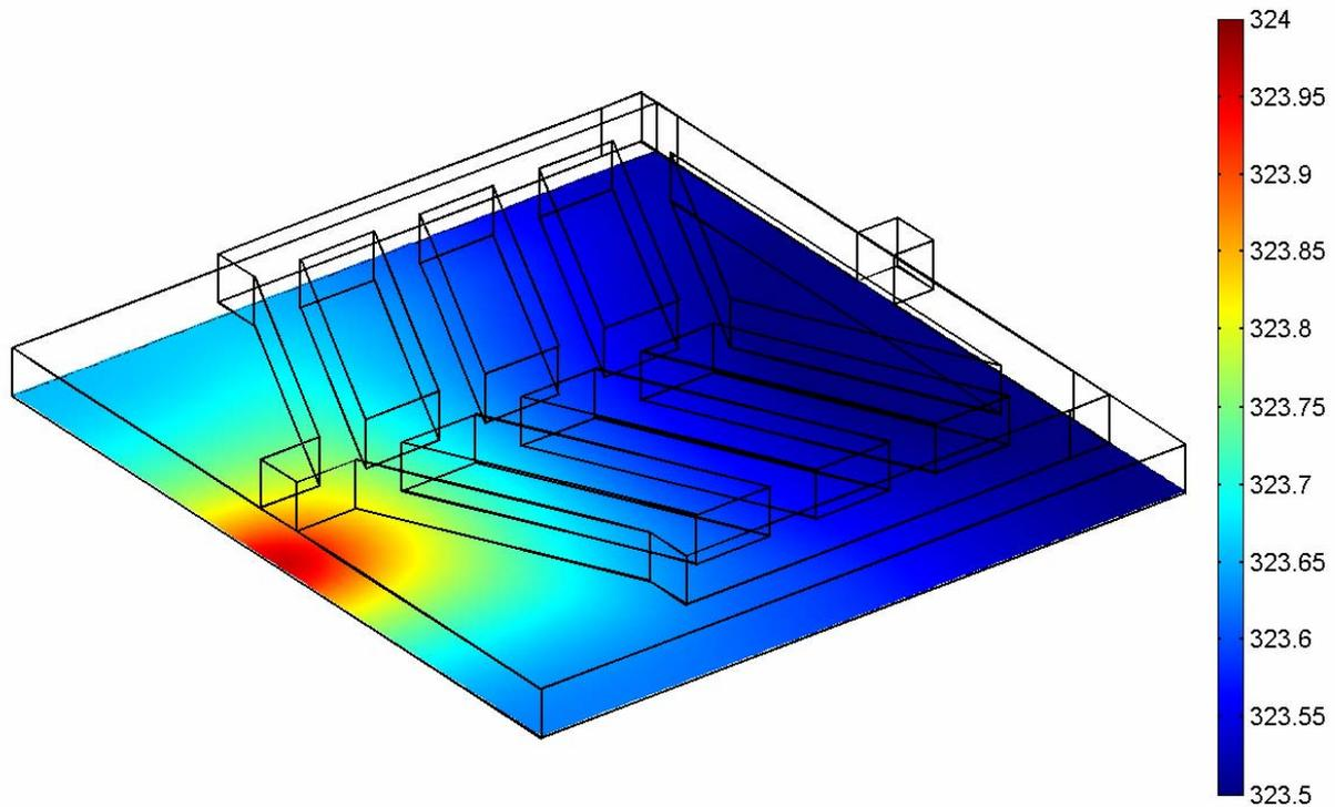
Figure 8. Temperature distribution at the cathode side catalyst layer.
