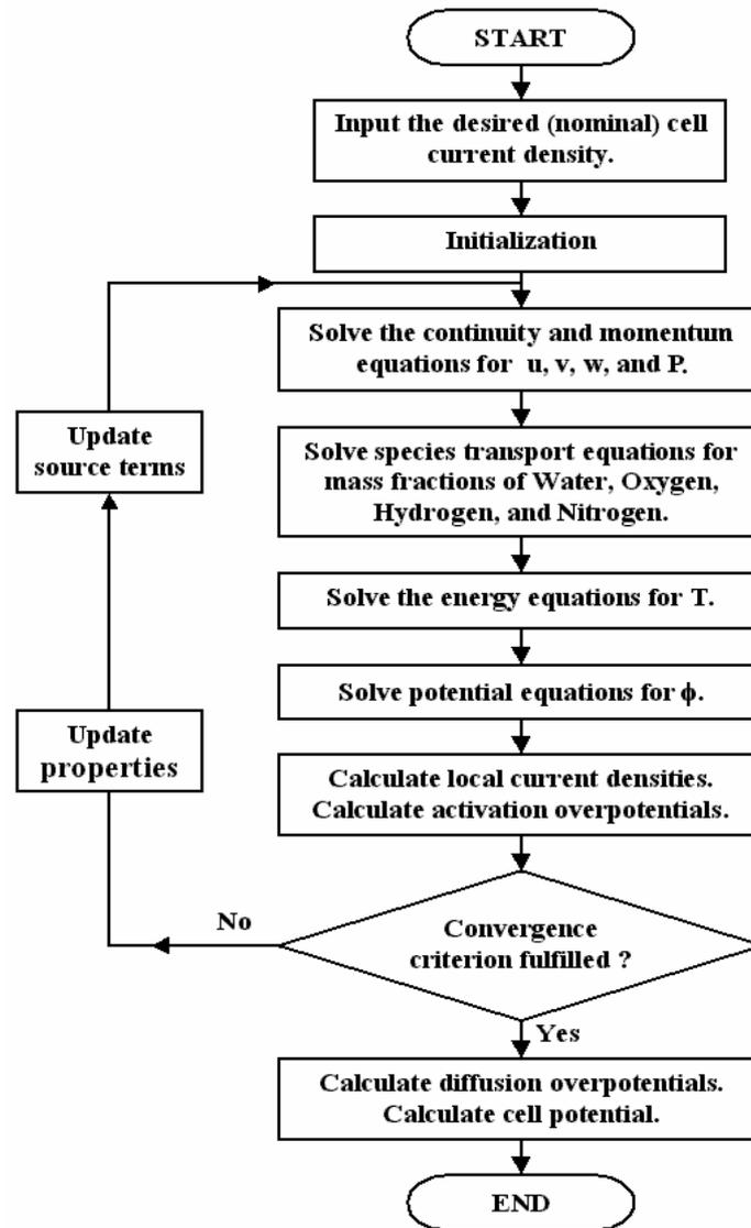
Figure 3. Flow diagram of the solution procedure used.
