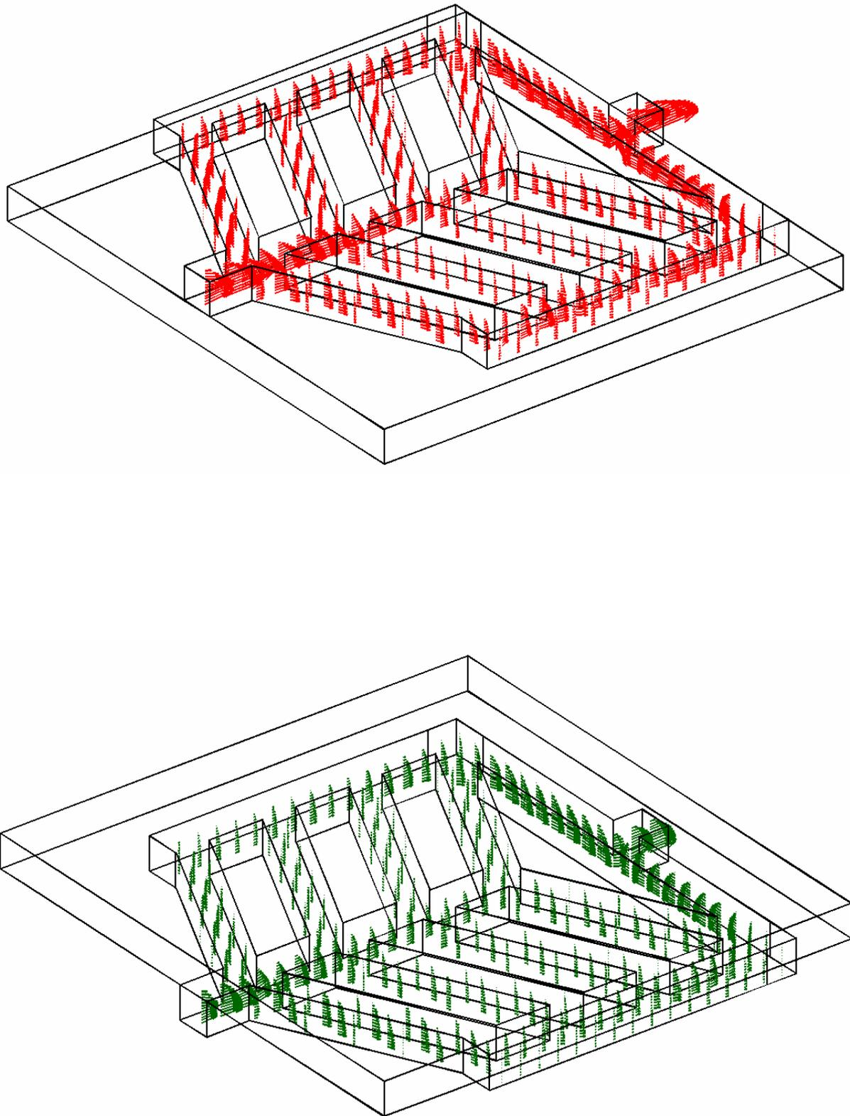
Figure 4. Velocity profiles in the mid-plane of the cathode (red) and anode (green) gas flow channels.
