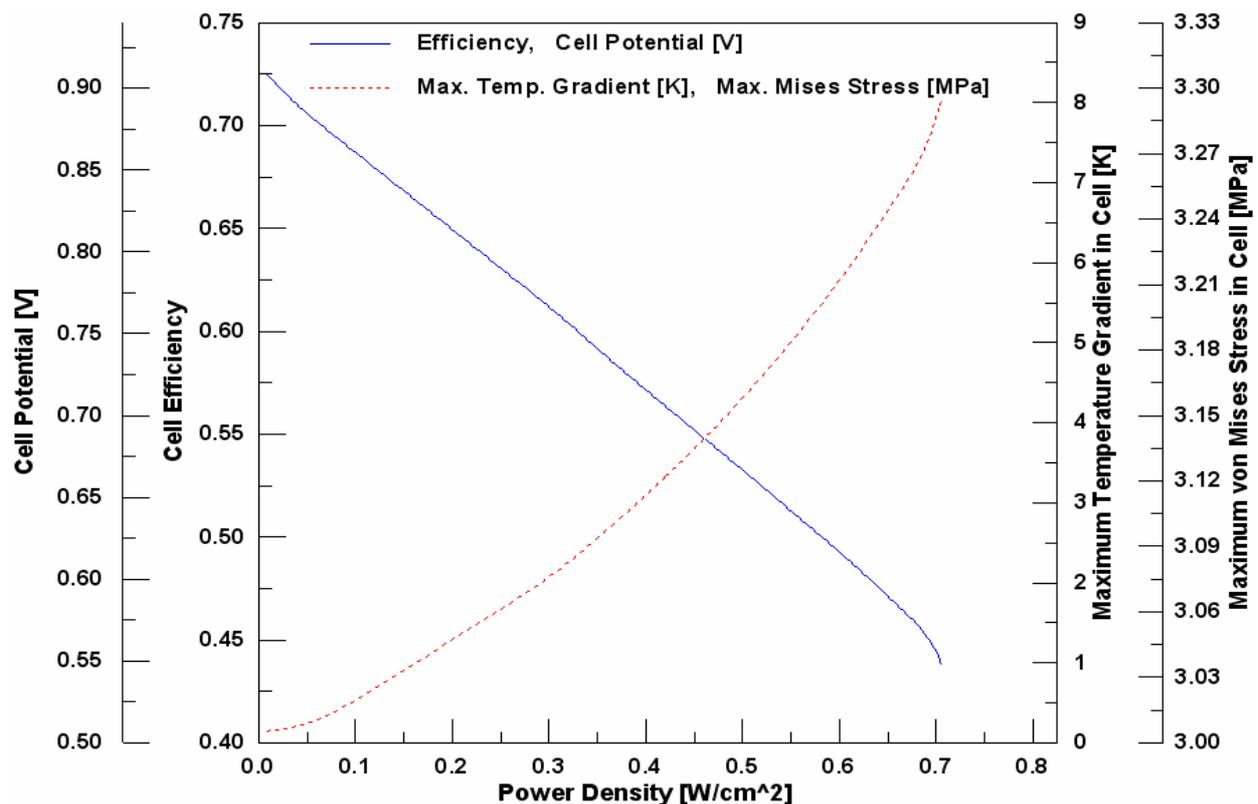
Figure 8. Relationship between the thermodynamic efficiency, the power density, and maximum stresses of the cell operates at base case conditions
