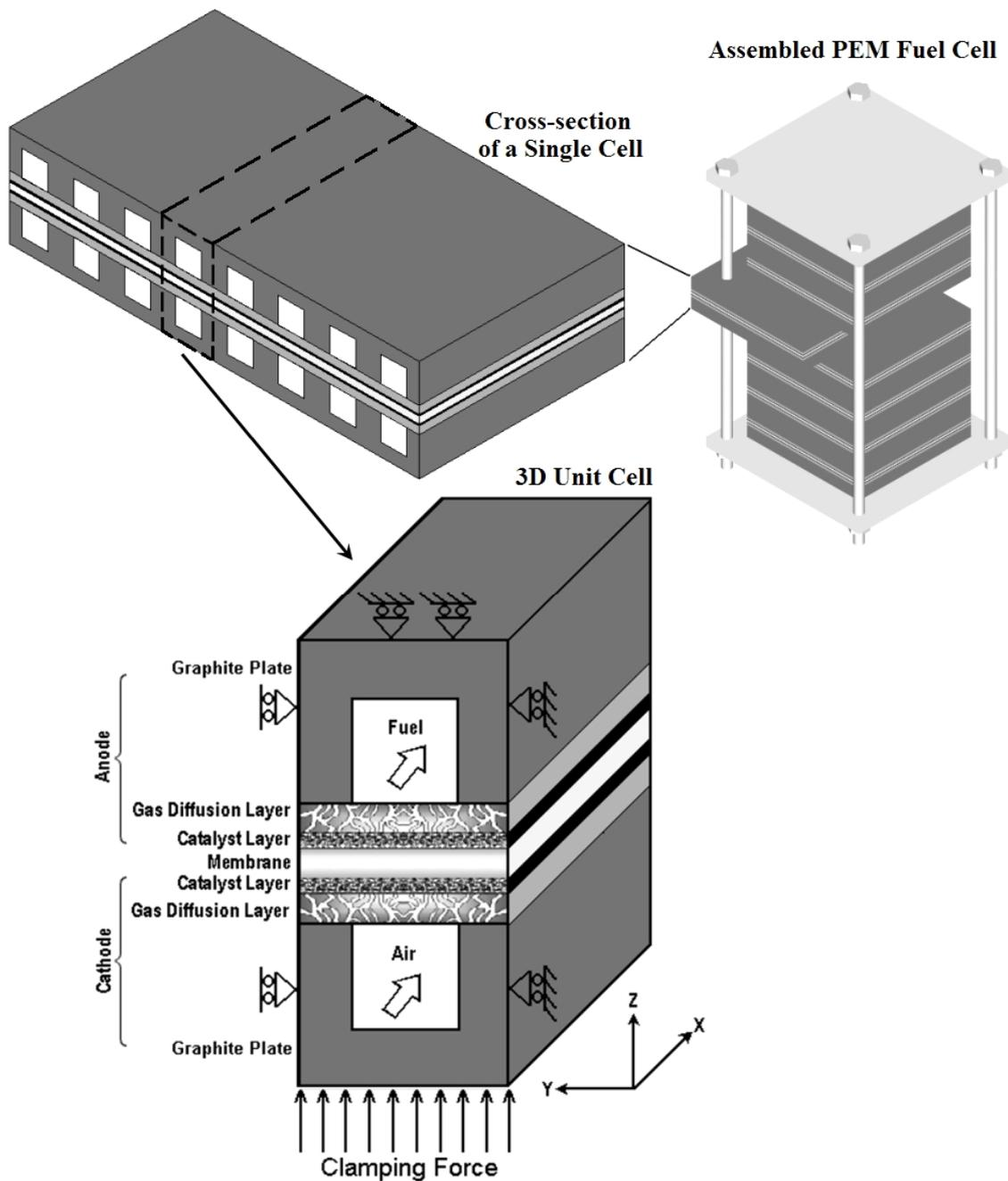
Figure 2. Three-dimensional computational domain
