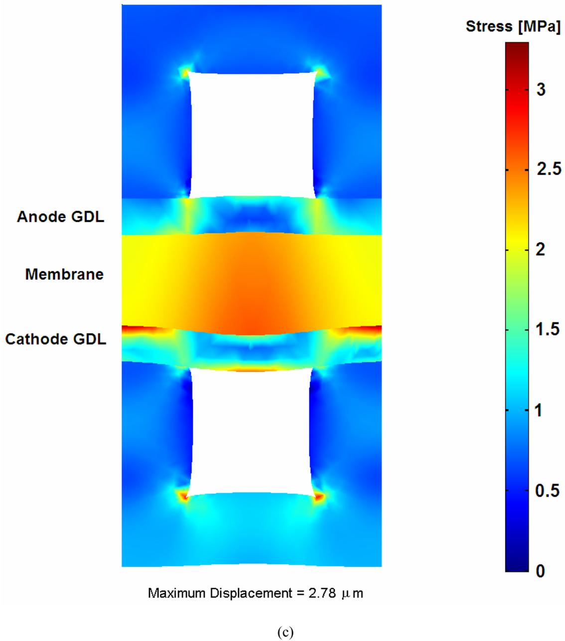
Figure 7. Von Mises stress distribution inside the cell (contour) and total displacement (deformed shape plot, scale enlarged 200 times) on the y-z plane at  $x=10$  mm for three different nominal current densities: (a)  $0.3 \text{ A/cm}^2$ , (b)  $0.7 \text{ A/cm}^2$ , and (c)  $1.2 \text{ A/cm}^2$
