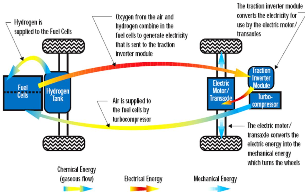
Figure 1. A zero-emission vehicle that utilizes a direct hydrogen polymer electrolyte fuel cell
