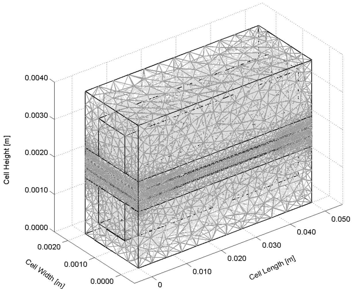
Figure 3. Computational mesh of a PEM fuel cell
