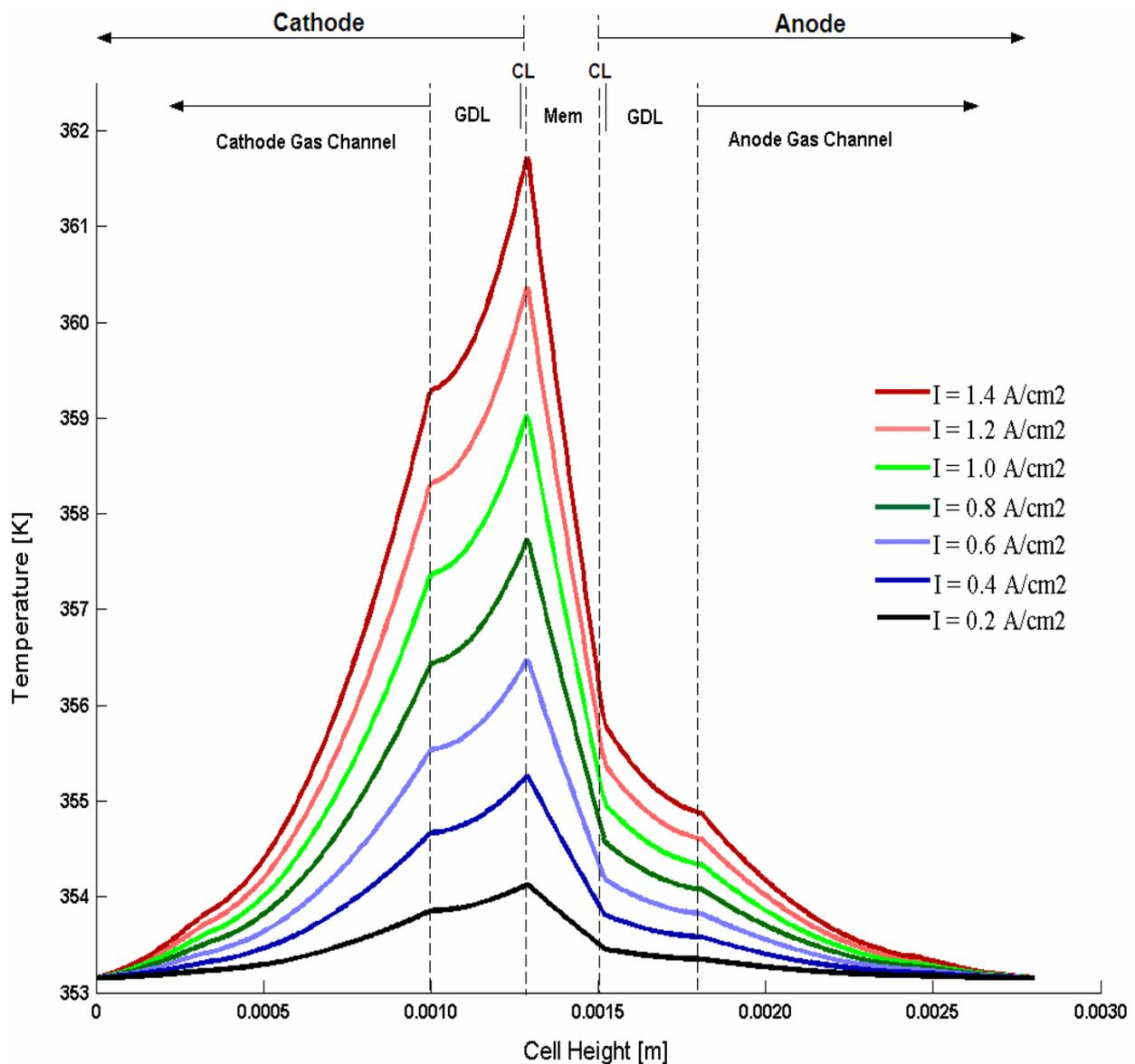
Figure 6. Temperature profiles along through-plane direction for multi-load conditions
