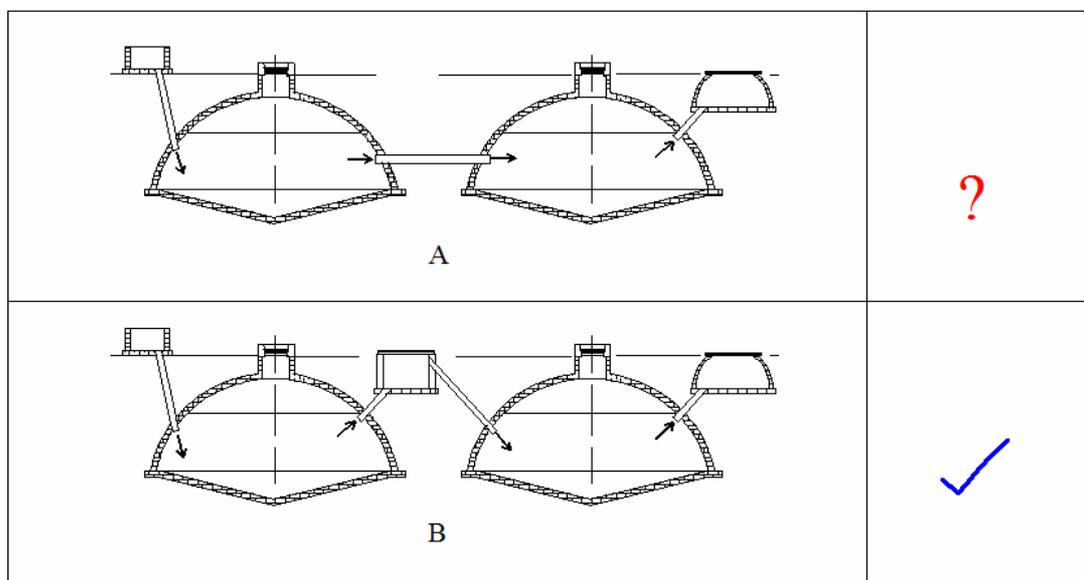
Figure 13. (A) Tandem digester layout used by BTWAL, BCEL, and BCL, and (B) Appropriate and recommended layout [23]
